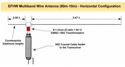
The EFHW antenna, shown above, indicates a 0.05 wavelength (7-foot-long) counterpoise. Typically this is omitted, as the coax braid serves that function.
