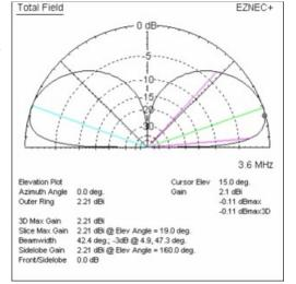
loss from ground absorption will be significant. These radial wires are untuned, so their length is not critical, though a quarter-wavelength is considered minimum. The installation effort for a vertical antenna lies mostly in its ground system - poor ground systems are common. An inadequate ground system adds considerable loss, especially at low angles. The penalty for a poor ground system could easily add 10 dB of attenuation. Your 100 watt transmitter now only radiates 10 watts!
