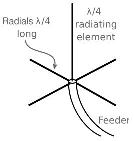
**Your takeaway:** If your vertical antenna lacks counterpoise radials, adding just one or two 32.5-foot radial wires to the coax braid at the base of the antenna may make a sustantial improvement in its efficiency. The counterpoise wires do not need to be symmetrical or look nice - just connect the wire and pull the opposite end to stretch it away from the antenna - in most any direction. In rooftop installations, laying the wires on or under the roof, or in a gutter, may be sufficient.
